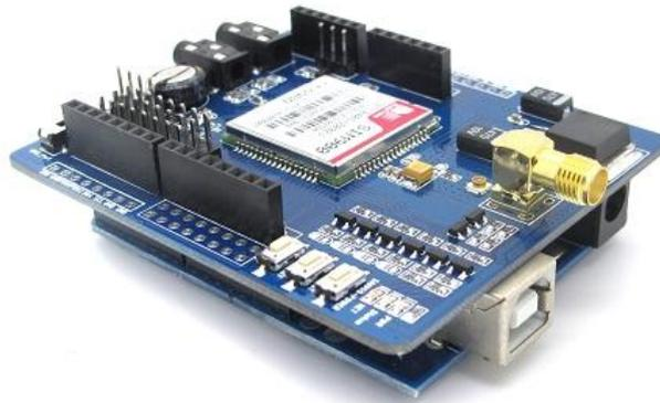
IComsat is a GSM/GPRS shield for Arduino and based on the SIM900 Quad-band GSM/GPRS module. It is controlled via AT commands (GSM 07.07, 07.05 and SIMCOM enhanced AT Commands), and fully compatible with Arduino / Iteadstudio and Mega.
