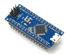
The Iteaduino Nano is a small, complete, and breadboard-friendly board based on the Adruino Nano 3.0. It has more or less the same functionality of the Arduino Duemilanove, but in a different package. It lacks only a DC power jack, and works with a Micro USB cable instead of a standard one.
