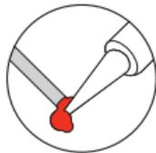
**Don't:** Glob the solder straight onto the iron and try to apply the solder with the iron.
